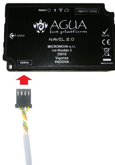
Figure 6. SERIAL cable and Wi-Fi module connection
